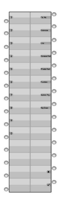
The keypad of the DSS28 unit consists of 28 programmable keys in 14x2 matrix structure, as shown in the illustration above. As can be seen in the illustration, the features that have been assigned to the keys in the beginning and that are supposed to be used upon entry to the programming mode are shown. In order for those features to be used correctly in normal and programming modes, 3 different functions have been defined. Uses of those functions have been explained below.
