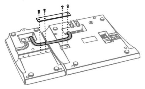
In order to maintain the physical connection between the DSS28 unit and the FT10/FT20 telephone set, the metal connection piece, which is included in the delivery package, must be fixed by the screws. There are connection points on Karel BT101 and Karel BT102 telephone sets, as well.
