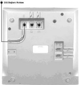
DSS25-28 Direct Station Select Module is connected to the DSS connection point on the ST26 and ST30 Digital Telephone Sets with the two-wire connection cable included in delivery package of the module.
