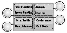
Each of the 16 keys in this group is used to activate any two of the operations by a single key, which have been stored in the memory.
