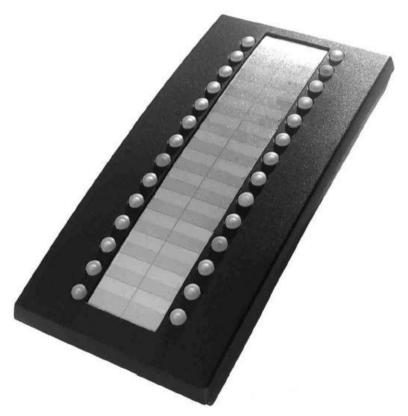
The Digital DSS25-28 Direct Access Unit consists of a keypad only. The keypad of the DSS25-28 unit is made up of 28 programmable, special-purpose keys and there is a LED available for each key. Functions that have been assigned to the keys can be monitored through those LEDs. The entire 28 keys are employed for assignment of access codes in general and there is no need for any programming over the unit.
