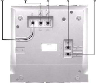
DSS CONNECTION: ST30 digital telephone set can be used with DSS25-28 module.
