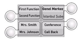
Two functions can be programmed for each of the speed dial keys, which consist of 16 keys with lights. Features that can be assigned to these keys through programming:
