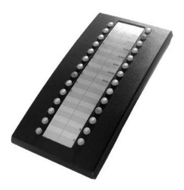
Digital DSS25–28 Direct Station Select Module consists of key pad. There are 28 programmable keys and a LED for each key. Functions of the keys can be followed by related LED. All of the keys are usually used to assign accessing codes, and there is not any necessity about programming on module.
